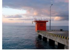
integrated concept was developed, which comprises three different tide gauge sensors and a GPS receiver for vertical control at each site. On-site, the data is quality checked and a detection algorithm for rapid changes in sea level monitors the station independently. All data are transmitted by using GTS/Meteosat and INMARSAT/BGAN. Solar arrays deployed on-site and different communication lines ensure an autonomous operation with minimal maintenance requirements.
